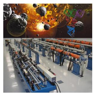
Panel 5. Prague Asterix Laser Systém (PALS) is a terrawatt iodine laser, which was used to simulate high-energy density processes. The laser shots simulated impacts of extra-terrestrial bodies into the early Earth's atmosphere simulant (Late Heavy Bombardment period). During this process, the formation of organic molecules (as complex as nucleic acid bases) from simple precursors (H<sub>2</sub>O, CO<sub>2</sub>, CH<sub>4</sub>, CO, N<sub>2</sub>) was discovered<sup>38,42-45</sup>
